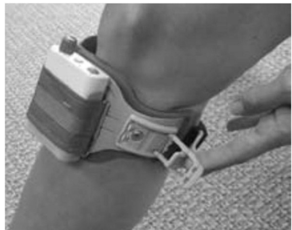
Fig. 1. Foot Drop Stimulator (WalkAide®, Innovative Neurotronics, Inc., Austin, TX, USA).
