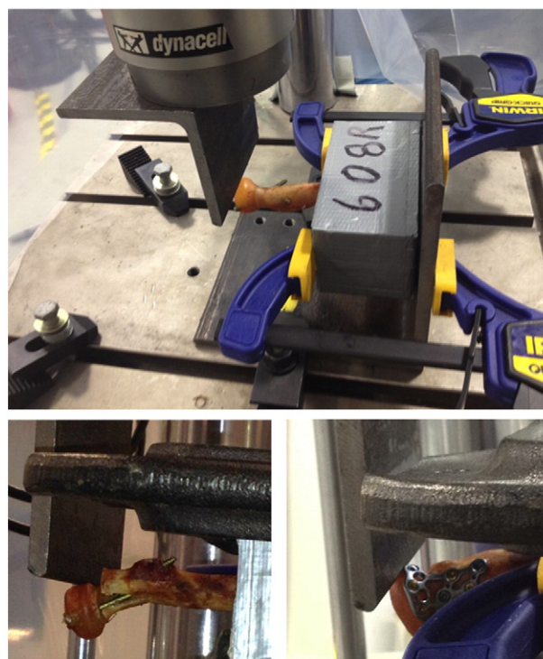
Fig. 2. Experimental setup for loading of radial head fixed with screws or plate in shear to failure in the PA direction.
