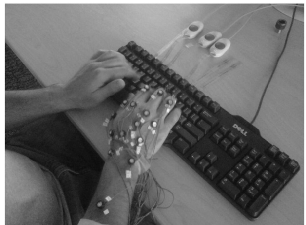
Fig. 1. Active markers affixed to the dorsal aspect of the dominant hand during the typing task.
