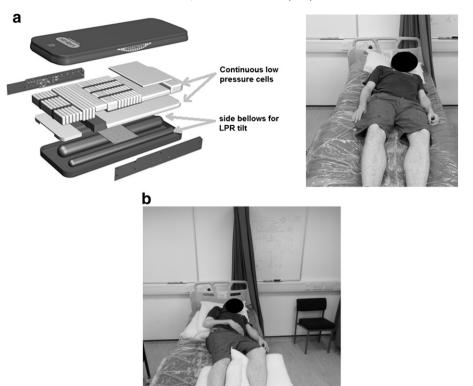
Fig. 1. (a) Schematic of the prototype LPR device with air billows to provide tilt. (b) Example of manual tilt to the left with the individual supported by pillows.
