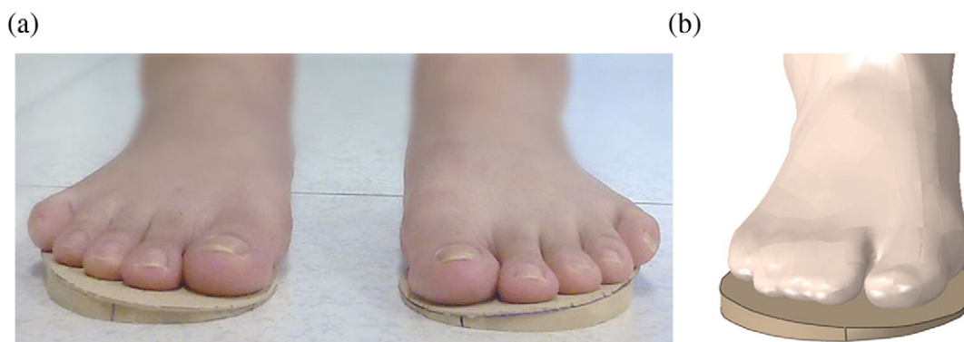
Fig. 1. The 5° LWIs investigated in this study. (a) The fabricated 5° LWIs used in motion analysis. (b) The developed 5° LWI in the FE model.
