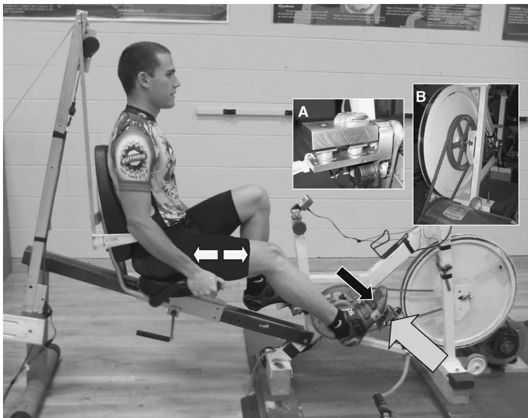
Fig. 1. Isokinetic eccentric cycle ergometer. Inset images show details of the instrumented force pedal (A) and motor driven flywheel (B). As the pedals move toward the participant (largest gray arrow), the participant resists by applying force to the pedals (black arrow at foot level). Because the magnitude of force produced by the motor exceeds that produced by the participant, the leg extensors (white arrows in thigh) actively lengthen (eccentric muscle action).
