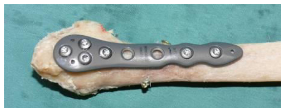
Fig. 3. Lateral plate. The construct includes an independent interfragmentary lag screw.
