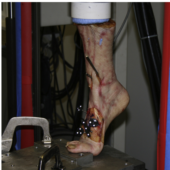
Fig. 1. A right foot specimen mounted onto the MTS machine. The ankle and subtalar joint have been fused with the foot in equinus. Steinmann pins used to strengthen the fusion are visible.
