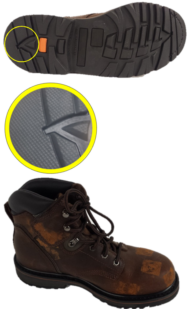
Fig. 1. Picture of tread pattern (top), heel region (middle) and boot upper design (bottom). The close-up view of the heel region is consistent with the circle marked on the top figure.
