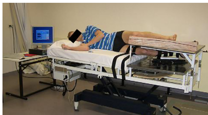
Fig. 1. Demonstration of positioning the subject on the Prosys. The right knee is tested while the left knee is held away at a second level.
