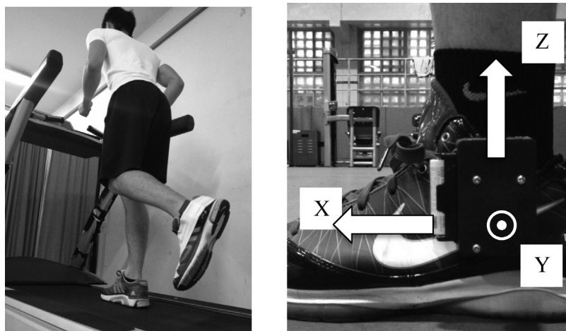
Fig. 1. The setting of IMU module and placement on the subject's left foot (left). Arrows represent anteroposterior (X) axis and superiorinferior (Z) axis, dot represent mediolateral (Y) axis (right).
