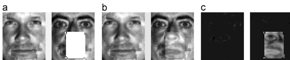
Fig. 1. Illustration of the low rank structure of occlusion error. (a) Observed images. (b) Recovered images. (c) Error images.
