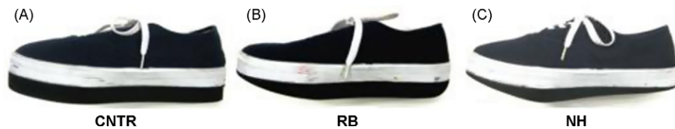
Fig. 1. Photographs of shoes showing control and experimental sole patterns: (A) control shoe (CNTR); (B) rocker bottom shoe (RB); (C) negative heel shoe (NH).
