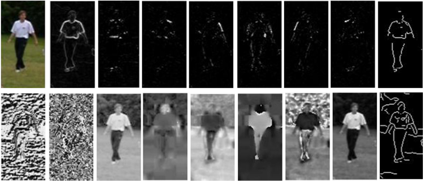
Fig. 1. Different channels of the input image (first row corresponds to the original, magnitude, gradient angle (6), sobel edge image; Second row corresponds to the LBP, orientation, LUV, HSV and canny image).
