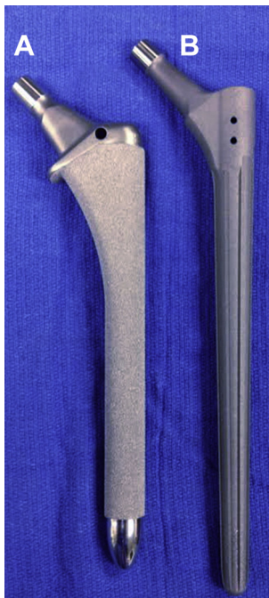
Fig. 1. (A) Zimmer Wagner SL Revision stem with 2° taper distal geometry and (B) Zimmer VerSys FullCoat Revision stem with cylindrical distal geometry.
