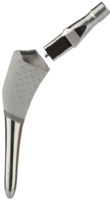
Fig. 1. The ABG II Modular stem system consists of a proximally hydroxyapatite (HA) coated titanium-molybdenum-zirconia-ferrite (TMZF) alloy stem with a cobalt-chromium (Co-Cr) modular neck segment with various options for neck length, version, and neck-shaft angle.
