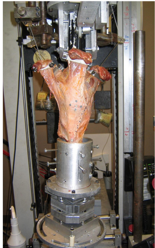
Fig. 1. Custom knee testing system with six degrees-of-freedom at both the femur and the tibia.
