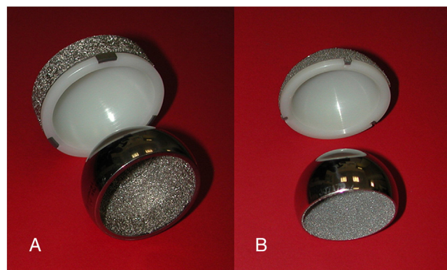
Fig. 1. Two different acetabular and femoral designs were utilized: (A) titanium fiber mesh acetabular component shown with a titanium fiber mesh femoral component and (B) titanium beaded acetabular component shown with a Co-Cr beaded femoral component.
