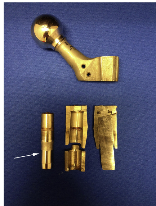
Fig. 2. The mid-stem modular junction of the reference, unfractured Revitan prosthesis after vertical sectioning. On the left is the CoCrMo cylinder connecting the proximal and distal components. In the middle, the surrounding proximal and distal components (with the CoCrMo cylinder removed). The distal component is fixed to the CoCrMo cylinder during the manufacturing, while the proximal component is attached intraoperatively. The arrow shows the level at which the fractures occurred in both cases.
