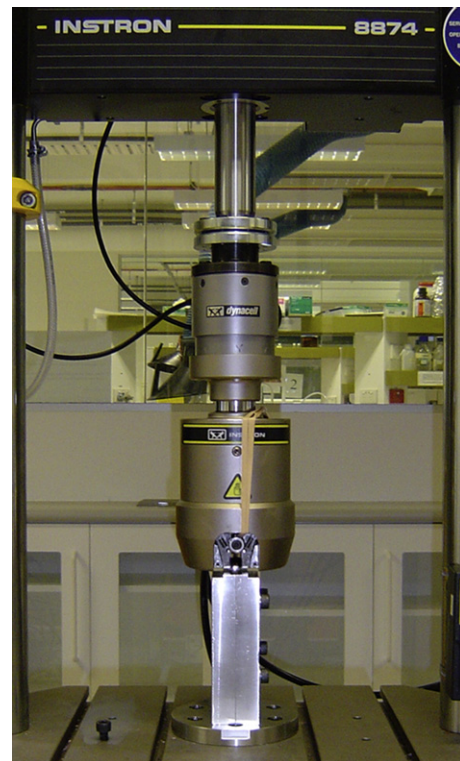
Fig. 2. Experimental setup pictured. Mounted to the base of the Instron is mold, which supports the cement mantle construct during testing.
