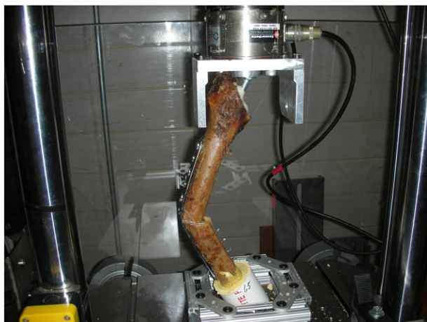
Fig. 1. Axial loading of cadaveric femur with proximal locking screw construct.
