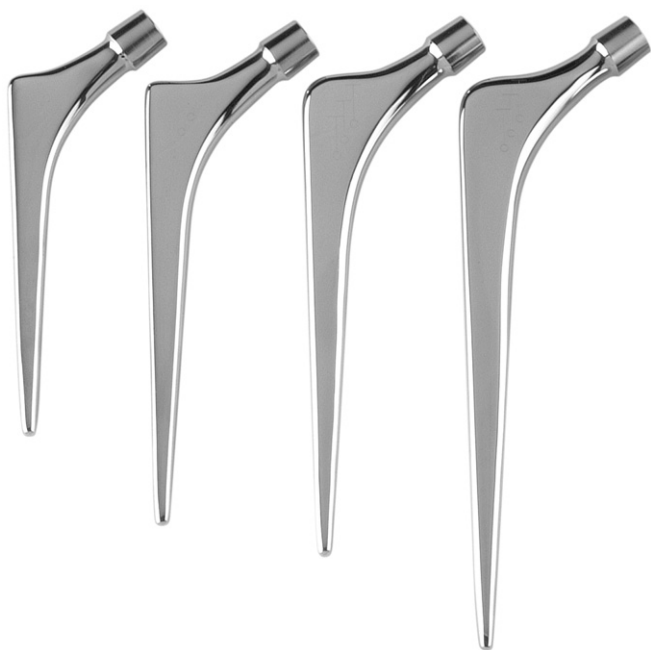
Fig. 1. Short and Standard Length Exeter Stems. Left to right: 95-mm length with 30-mm offset, 115-mm length with 33-mm offset, 125-mm length with 35.5-mm offset, and 150-mm length with 37.5-mm offset.
