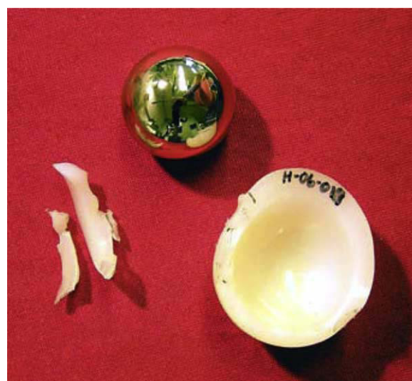
Fig. 2. The Marathon UHMWPE explanted acetabular liner, along with pieces of its broken rim and its femoral head.
