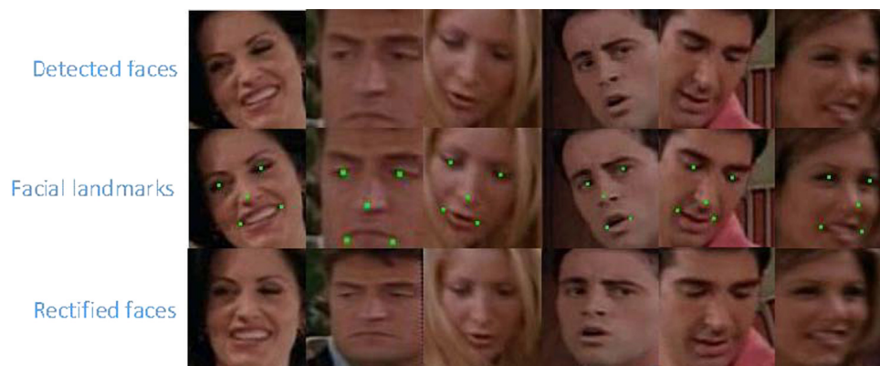
Fig. 2. Face rectification by the facial landmarks. The three rows from top to bottom are the original detected faces, the detected faces with landmarks and the rectified faces.
