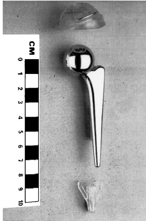
Fig. 2. Sheep THA prosthesis comprising a Corethane CL acetabular component, a stainless steel double-taper femoral component, and a plastic centralizer.
