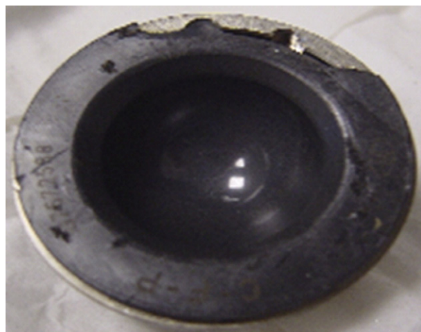
Fig. 2. The composite liner and metal cup were firmly secured in position with the PEEK locking ring. A portion of the cup's rim was broken away during surgery.
