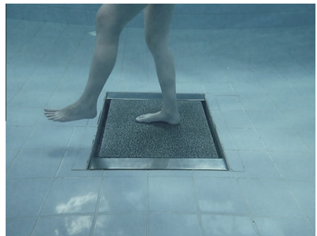
Fig. 1. Underwater force platform during data collection.
