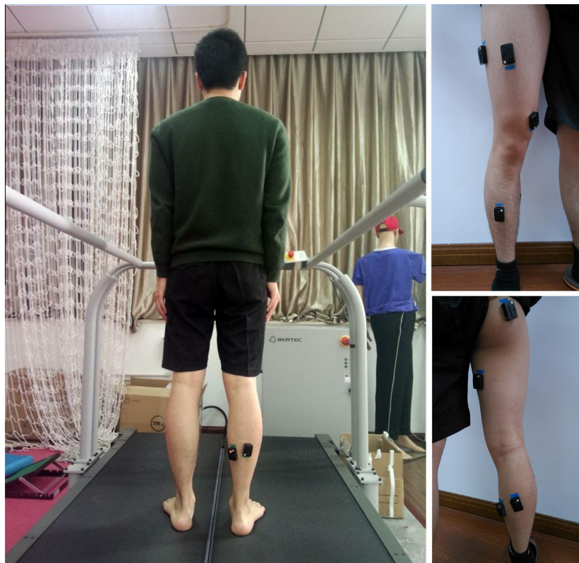
Fig. 1. The experimental setups. Eight EMG sensors are attached on the positions over target muscles of the legs.
