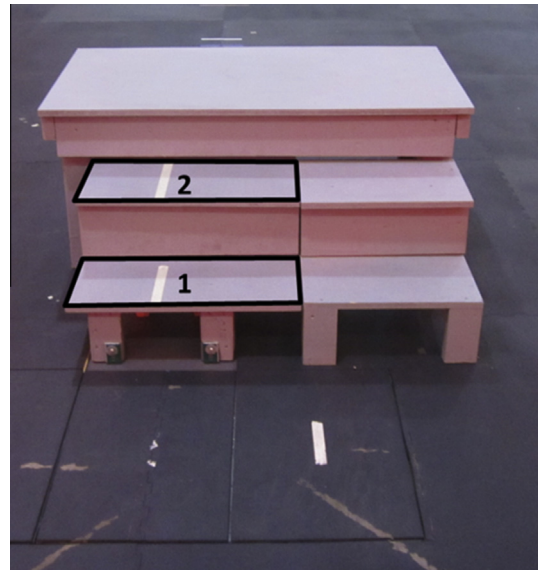
Fig. 1. Stair Setup. The first and second steps, in the identified areas, are instrumented. The peak angles and moments during stance were measured on step 2 during ascent and step 1 during descent.
