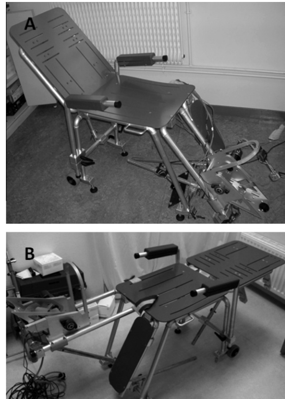
Fig. 1. Ergometric device and its foot-plate in seated (A) and supine (B) positions.
