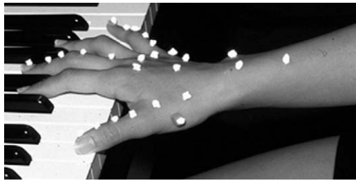
Figure 1. Twenty-six reflective markers, 2 mm in diameter, were placed on the dorsal side of the fingers, hand, and distal forearm for 3-dimensional motion analysis (Expert Vision System).
