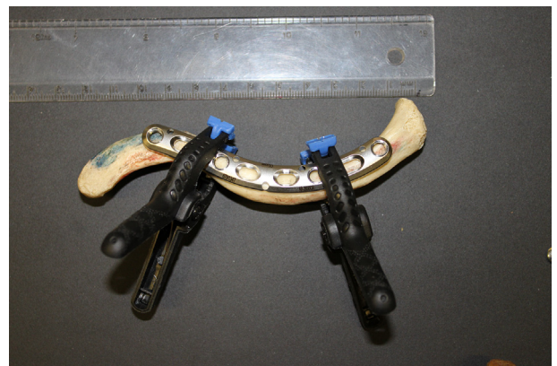
Figure 1 A superior middle clavicle plate attached to a clavicle via 2 plastic modeling clamps.
