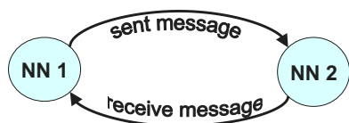
Fig. 1. The classical asynchronous point-to-point one-directional message passing between two locations that hold a different neural network classifier.
