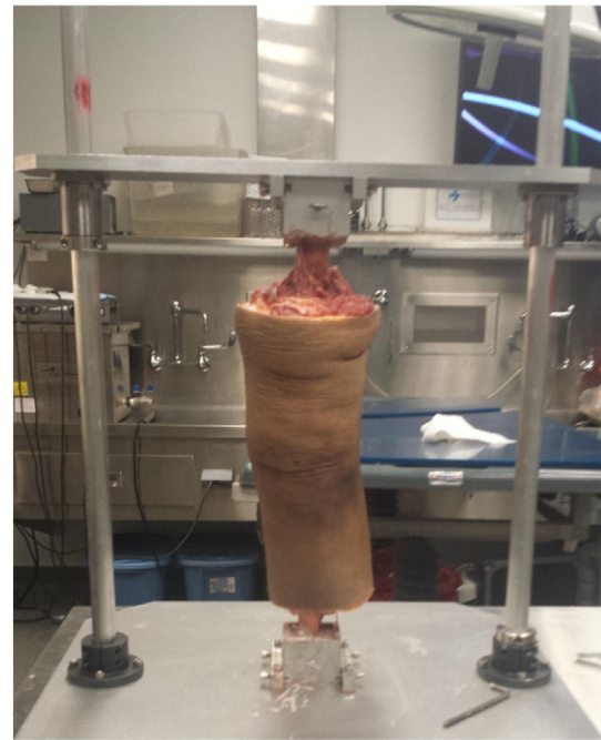
Figure 1. Example specimen placed in the mechanical load frame in unloaded condition ready for ultrasound.
