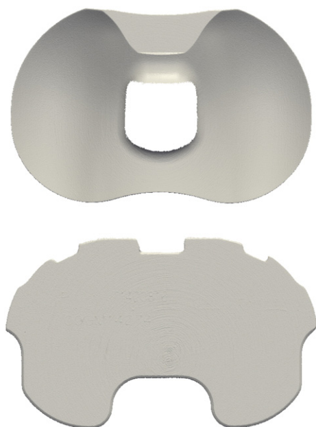
Fig. 1. The extracted articular (top) and backside (bottom) surfaces from the 9 mm thick intact tibial insert.
