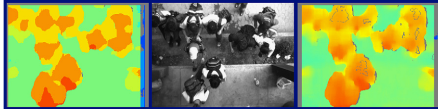
Fig. 2. A dense scene (center) captured from above and two corresponding range images. The student's heads appear at the darkest spots in the blobs. The right image was extracted using sub-pixel interpolation and has higher range resolution.
