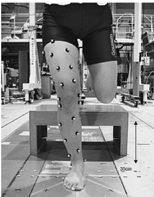
Fig. 1. Landing position and arrangement of makers. Subjects performed a single limb drop landing from a 30 cm platform. Twenty four reflective markers of 9 mm diameter were secured to the limb.
