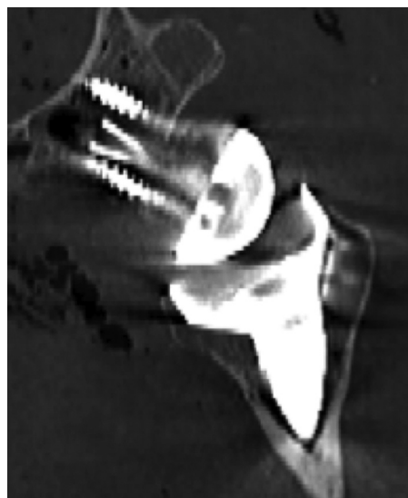
Fig. 2. A coronal CT image of a specimen with a 4 mm simulated resorption gap, which was incorrectly reported by both observers as having no gap (0 mm).
