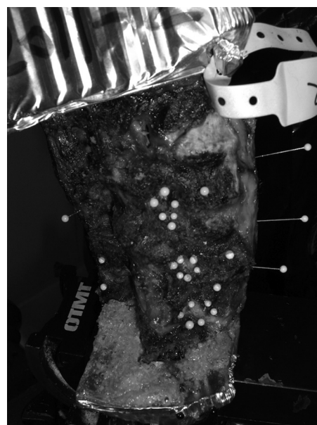
Fig. 2. Six markers were placed around each of the three foramina of interest, namely, L3–L4, L4–L5, and L5–S1. The stereoscopic cameras record the changes in spatial position of these markers, in flexion and in extension, thereby enabling measurement of the changes in foraminal surface area.
