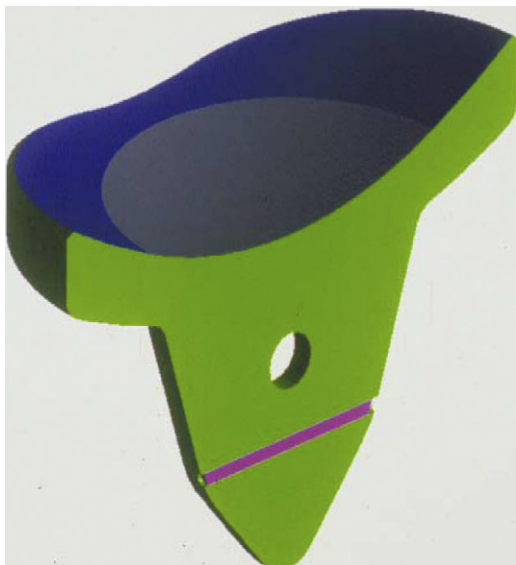
Figure 2 Dual-radius glenoid implant with central conforming zone and peripheral nonconforming zone. (Color version of figure is available online.)
