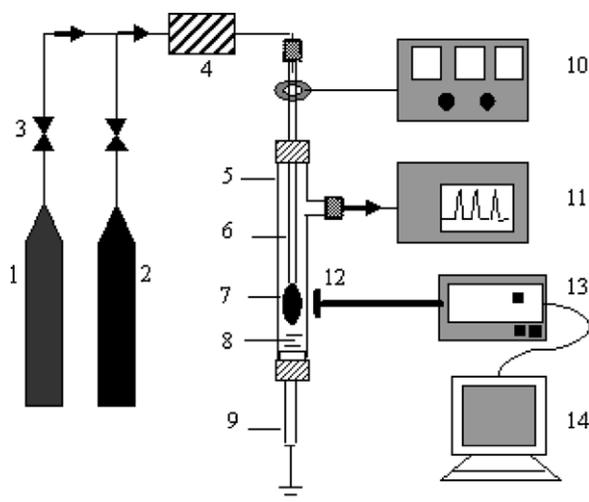
**Fig. 1.** Schematic diagram of the plasma apparatus. (1) methane, (2) hydrogen, (3) mass flow controller, (4) mixture, (5) quartz tube, (6) plasma powered electrode, (7) plasma zone, (8) ionic liquids, (9) grounded electrode, (10) DC plasma generator, (11) gas chromatography equipment, (12) optical fiber, (13) OES, (14) computer.
