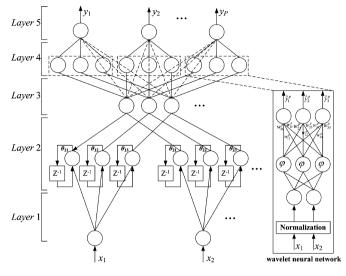
Fig. 1. Schematic diagram of RWNFS model.
