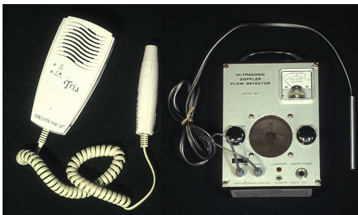
Fig. 1. Handheld acoustic Doppler ultrasound devices. Left, 5-MHz vascular probe (Medasonics, Newark, CA) used daily in our office practice; right, Ultrasonic Doppler Flow Detector with 8.9-MHz probe (Model 811-B, Parks Medical Electronics, Inc, Aloha, OR) native to our operating rooms and hospital floors.
