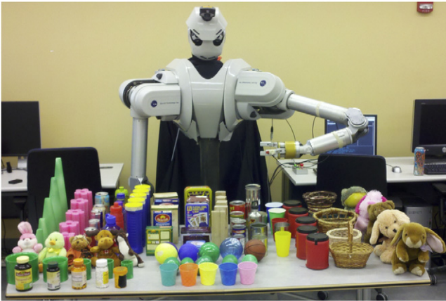
Fig. 1. The humanoid robot used in our experiments, along with the 100 objects that it explored.
