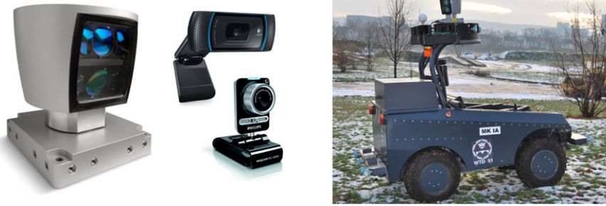
Fig. 1. Deployed sensors and robot: A 3D laser range finder and two different commercially available cameras are used to perceive the environment. Sensors are mounted on top of a 500 kg outdoor robot.
