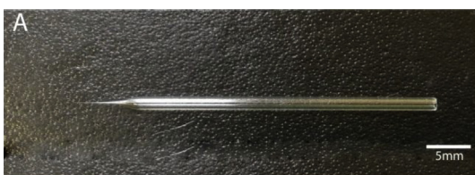
Fig. 1. The length of the glass electrode.
