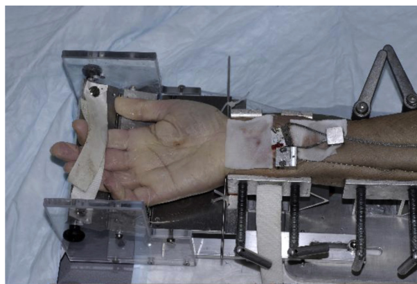
Figure 1 Custom-made jig for the arm to secure its position.
