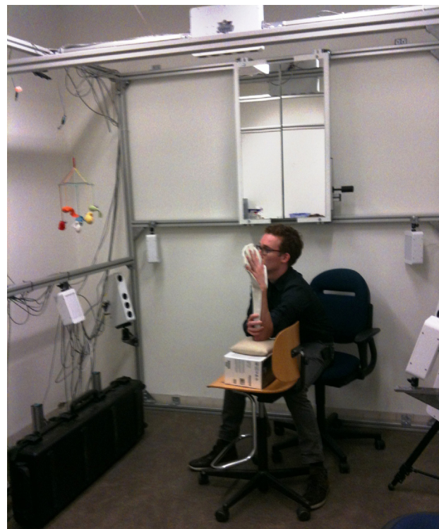
Figure 1 3D stereophotogrammetrical camera alignment. Legend: 3D stereophotogrammetrical camera alignment, with the hand positioned in the center and the template in place.
