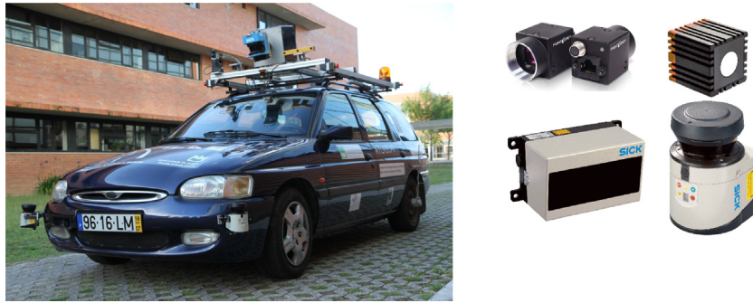
Fig. 1. ATLASCAR, a Ford Escort SW 98 adapted for autonomous driving capabilities on the left. Sensors used in this work—Sick LMS151 and LD-MRS40001, Point Grey camera and SwissRanger—on the right.
