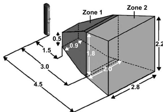
**Figure 1** Measurement volume of the OPTOTRAK PRO 1000<sup>®</sup> (Northern Digital Inc., Ontario, Canada) is shown. The camera is on the left. The optimal measuring distance between object and tracking camera is 1.5–3 m in zone 1. These distances are adapted to the demands of our operating theatres.
